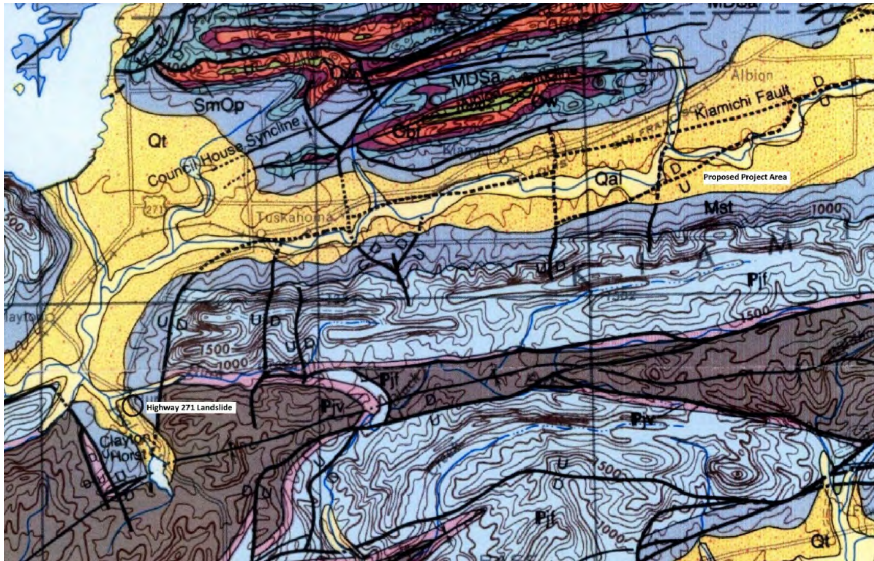
Figure 10. Part of the geologic map of Pushmataha County and surrounding areas by Marcher and Bergman (1983), with the area of the landslide along U.S. Highway 271 described by Nevels (2010) shown by the small black circle in the lower left-hand part of the figure. The area of the proposed Project is south of the town of Albion and the Kiamichi River in the upper right.
