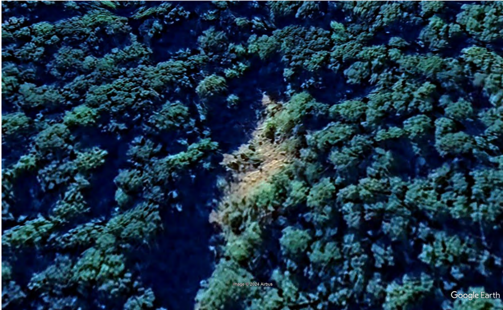
Figure 11. Google Earth image, looking southward, of a recent slope failure within the proposed site of the Pushmataha County Pumped Storage Hydroelectric Project, about 1½ miles south of the Kiamichi River and about 3½ miles south of the town of Albion. The failed slope is about 80 feet wide, from west to east, and about 180 feet long.
