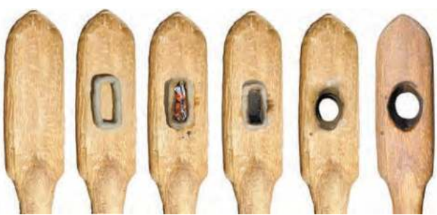
Fig. 6: Process of burning out a mortise to receive the ax head.
