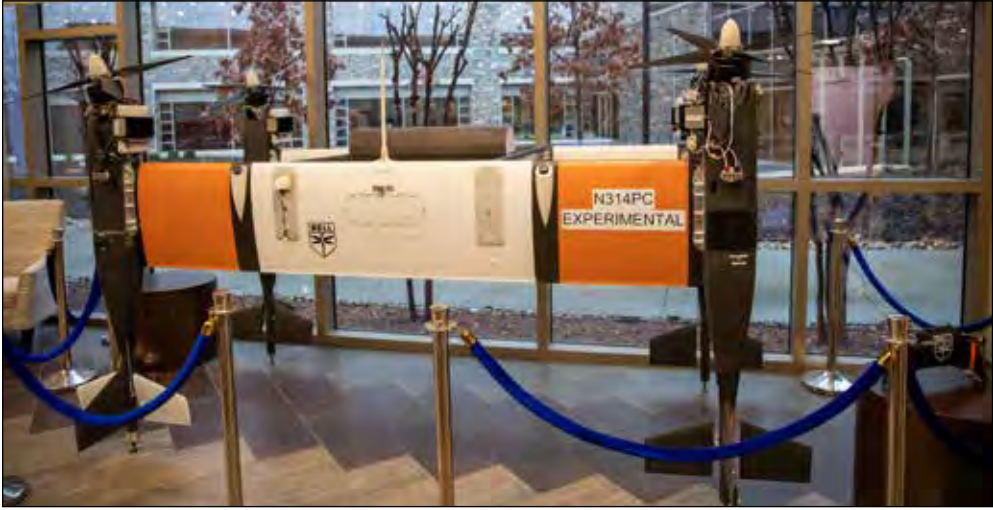
One of the drones used by Bell Textron Inc. in partnership with the Choctaw Nation’s drone program. This particular drone can carry up to 70 pounds and has a flight speed of 100 miles per hour.
